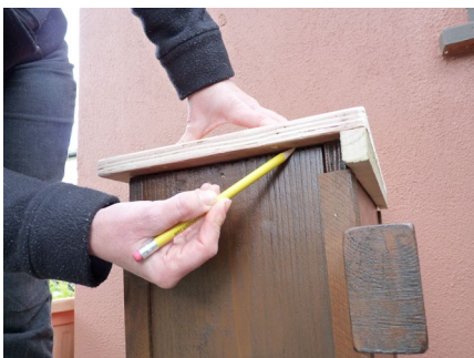
16. Test fit this onto the box and scribe a line using a pencil to show the position of the front and sides of the box.
