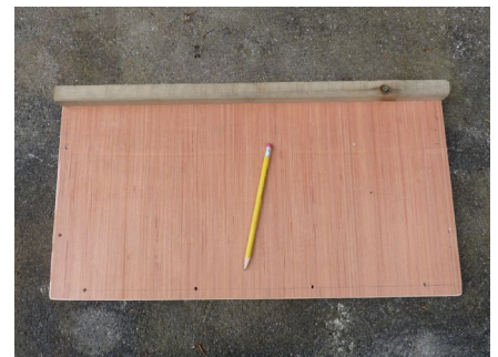
15. Screw the rear batten to the underside of the lid.
