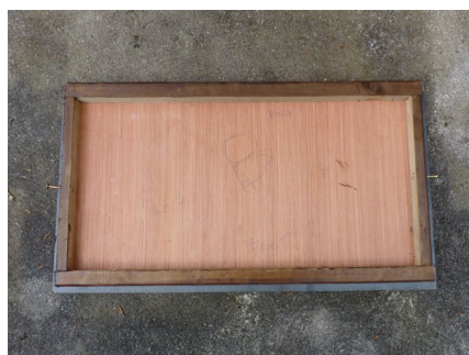
17. Fit the remaining battens, ensuring that the fit on the box is snug.*
